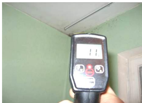
3. Photos. Examples of thermal bridges and low quality of indoor climate in Seminari street buildings.
